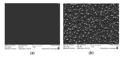
**Figure 2.** Morphology of: (**a**) TiO<sub>2</sub> magnetron sputtered coating on glass substrate (×5000); (**b**) TiO<sub>2</sub>/Ag<sub>23.1 at.%</sub>/Cu<sub>21.6 at.%</sub> magnetron cosputtered coating on glass substrate, Sample 5.
