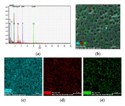
**Figure 1.** EDX spectrum (**a**), integrated map of Ti, Ag and Cu distribution (**b**) and maps of the individual elements Ti (**c**), Ag (**d**), Cu (**e**) distribution in Sample 5—TiO<sub>2</sub>/Ag<sub>23.1 at.%</sub>/Cu<sub>21.6 at.%</sub>.
