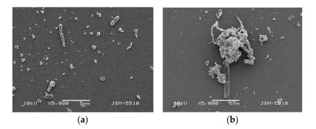
**Figure 6.** SEM images of significantly damaged *E. coli* cells (**a**) and *E. coli* cell aggregates (**b**) in contact with  $TiO_2/Ag_{23.1 at.\%}/Cu_{21.6 at.\%}$  magnetron cosputtered composite coating.
